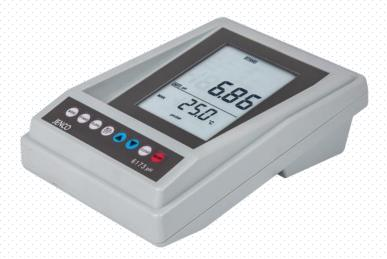
pH/mV/Temperature benchtop meter with an extra large LCD display for ease of use. Features a splash proof and rugged case ideal for schools and universities. Features Electrode Efficiency Function, multiple buffers 4.00, 4.01, 6.86, 7.00, 9.18 & 10.01 and automatic slope, buffer and electrode offset recognition. Has power down memory backup and works on 6 AA batteries or 100  $^{\sim}$  240 VAC adapters. CE Approved & ISO 9001 Certified.
