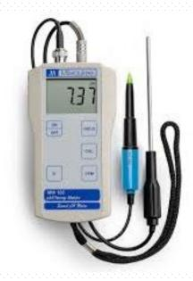
The Milwaukee MW102 + Food pH meter has won fans around the world with its reliable, fast and simple operation as well as its toughness and accuracy. The MW102 Food pH meter combines the power of the MW102 meter with the specialist capabilities of the MA920B/1 Direct Measurement Food Grade pH Probe.
