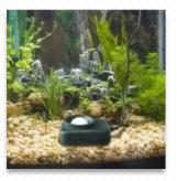
Put the light sensor on a stable surface in the aquarium, and hold the meter at a proper distance to avoid any interference or disturb to the sensor illumination.
