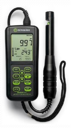
•Logging Memory: Up to 1,000 log records (stored in up to 100 lots) | On demand, up to 200 logs | on Stability, up to 200 logs | Interval logging, up to 1,000 logs | Parameter-Specific log storage location
