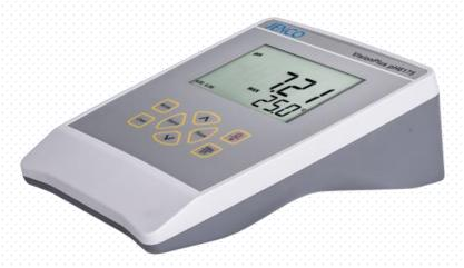
Jenco 6175 benchtop pH meter is the successor of the popular 6173 benchtop pH meter. While the large LCD display and easy of use remains firmly in place, model 6175 now offers 0.1 mV resolution for ISE applications and a streamlined look. This pH benchtop is RoHS compliant.
